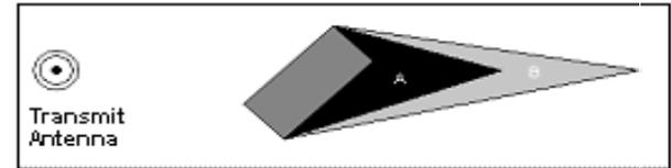
Figure 1.1 – Shadowed areas due to structures
