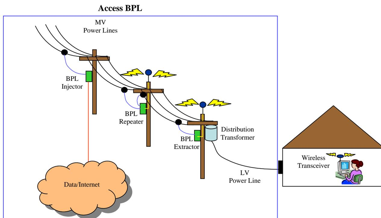
As shown in Figure 2, the hybrid Access BPL system uses repeaters and extractors which are capable of transmitting and receiving wireless signals to and from end-users.
